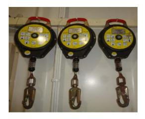
Picture of Fall arresting device used on board
