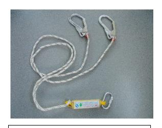
Lanyard with shock absorber shall be connected to safety harness.
